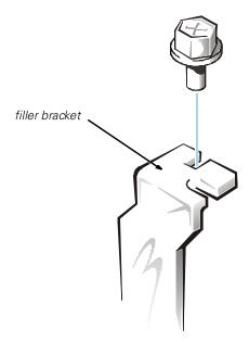
Figure 8-2. Removing the Filler Bracket
